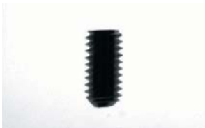
Direct Backlight (MDBL-CB70) Shape unclear because of stray, direct light.
