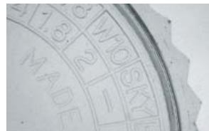
Direct Backlight (MDBL-CB70) Ordinary light transmitted evenly through the entire object.
