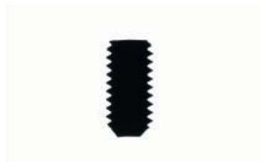
Collimated Backlight (MCBP-CB3430) Easy to identify shape because effect of stray, direct light is eased by the Collimated light.
