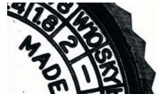
Collimated Backlight (MCBP-CB3430) Reflected light directed at characters for clear identification also makes external shape identification possible.
