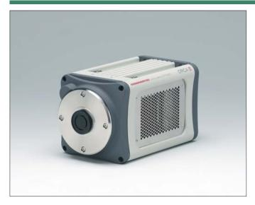
The ORCA II has a specialty feature of low noise and high-sensitivity. Maximum cooling down to -90  $^{\circ}$ C enables dark current as low as 0.0012 electrons/pixel/second and the 1024  $\times$  1024 pixels BT-CCD (Back-thinned CCD) provides 1M pixel resolution and high quantum efficiency of over 90  $^{\circ}$  peak and broad sensitivity from UV to NIR. This camera is especially suitable for applications which require to detect faint light with long exposure time and low noise.
