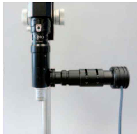
Köhler Illumination is recommended for objectives with magnifications higher than 20x
